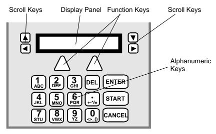
Figure 4. Keys on the Keypad
